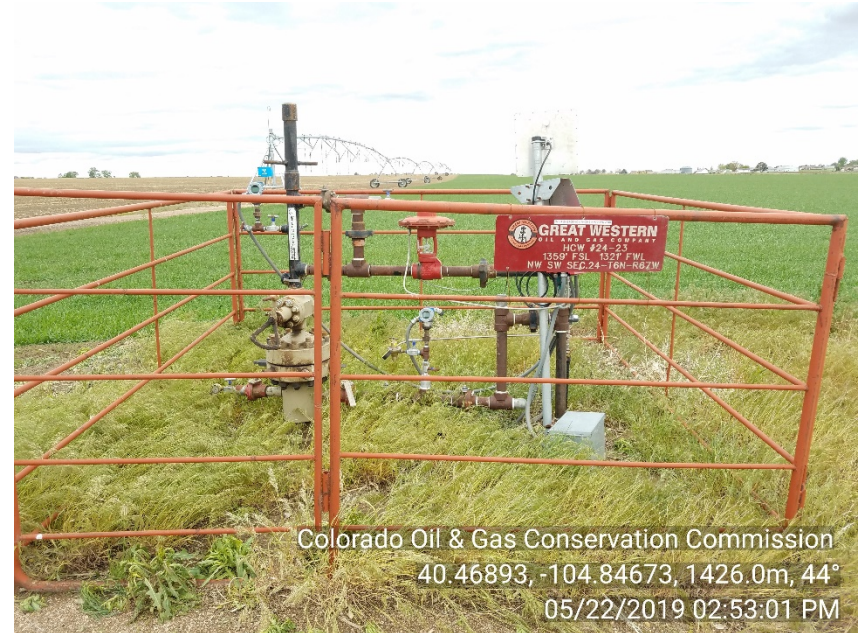
Photo #4 HCW 24-23 Wellsite Shut-In | SI Emergency number NOW posted Sign attached
