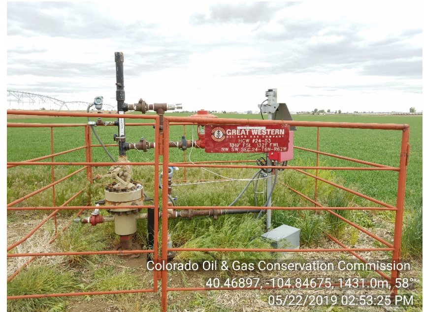
Photo #6 HCW 24-53 Wellsite Shut-In | SI Emergency number NOW posted Sign attached
