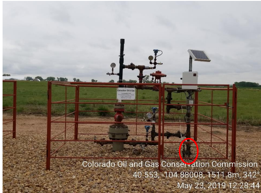
Photo 1: Wellhead; UNUSED RISER
