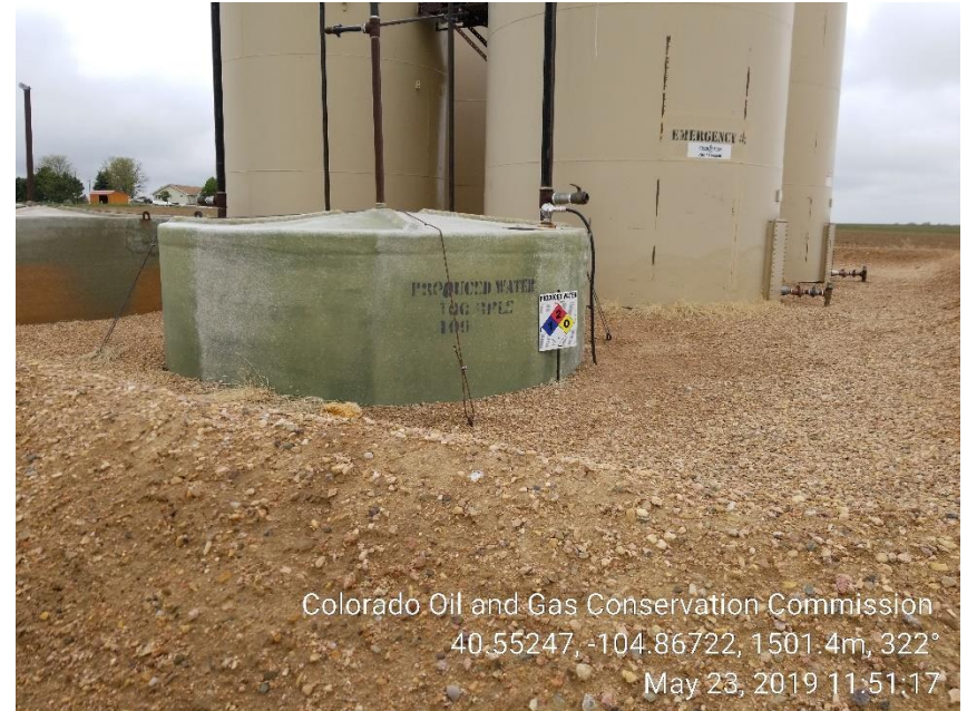
Photo 4: Not legible BBLS on produced water tank
