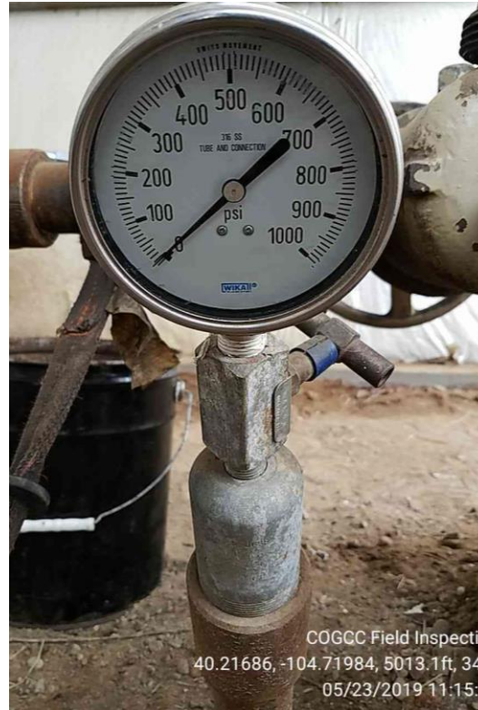
Photo 2 Bradenhead Gauge at start of test
