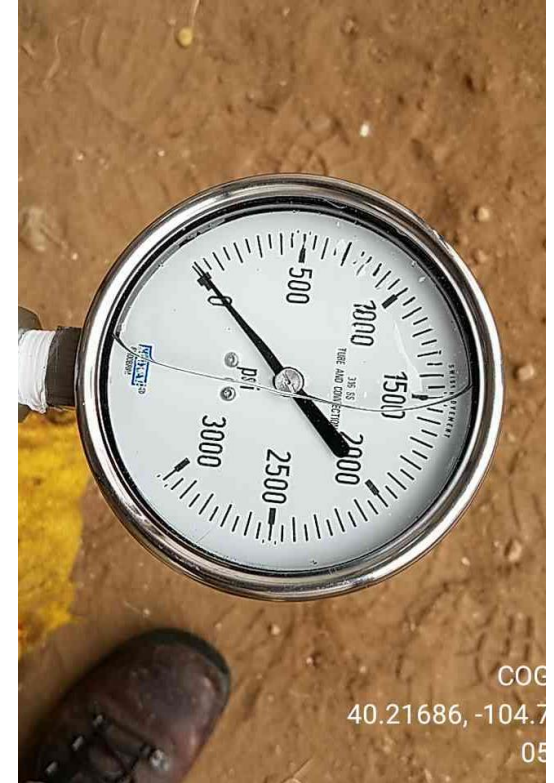
Photo 3 Casing Pressure at start of test
