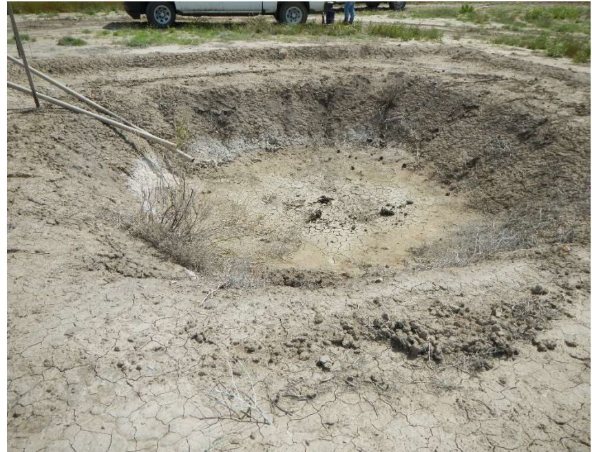
Photo #2 – View of the pit looking east. Weeds can be seen growing in and around the pit. The disturbed area at the base of the pit is where the operator collected their soil sample.
