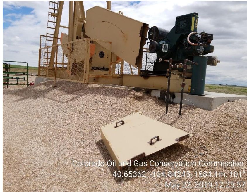
Photo 7: Door off pumpjack motor.
