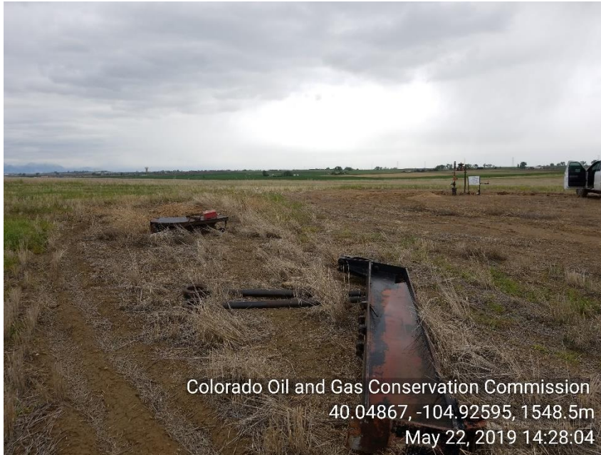
Photo 3 Unused equipment: Walking beam and horses head laying on location.
