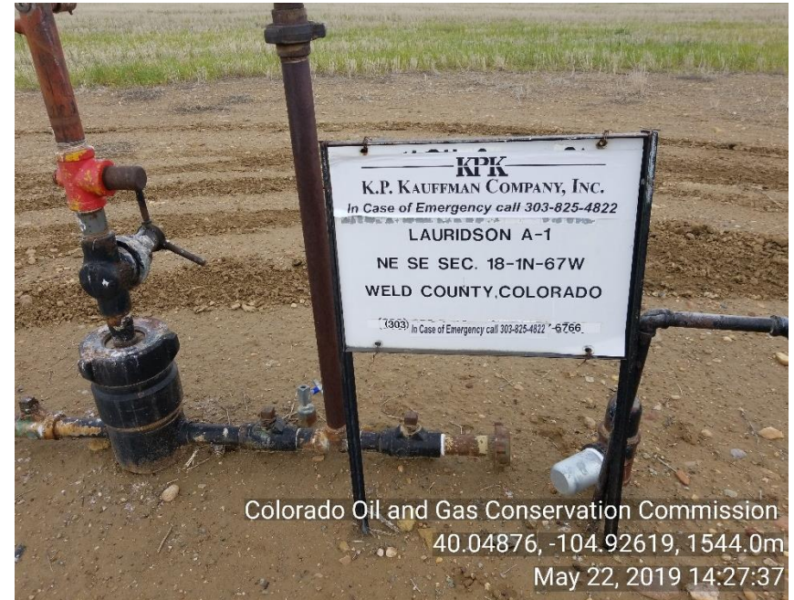
Photo 2 Production line not connected and bull plugged
