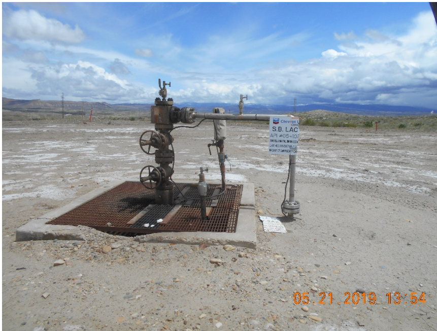
Injection wellhead
