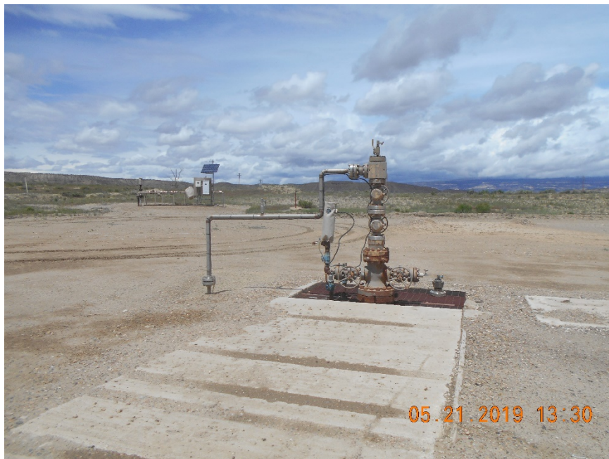
Injection wellhead
