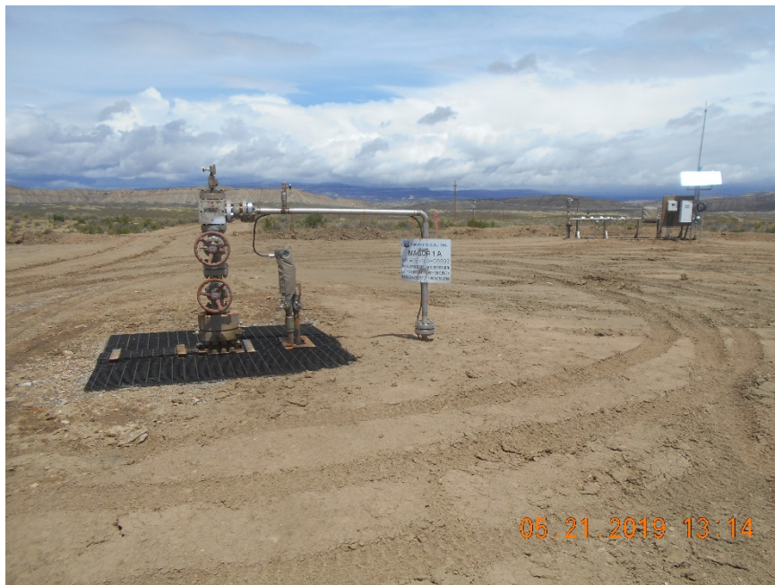
Injection wellhead
