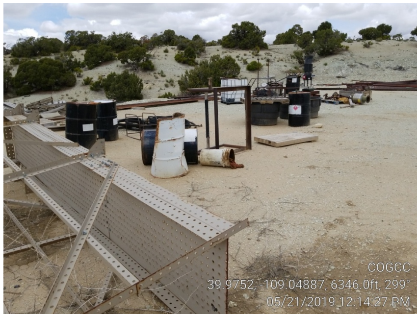
Photo 2. Assortment of trash stored mixed in with usable equipment. Barrels with no secondary containment.
