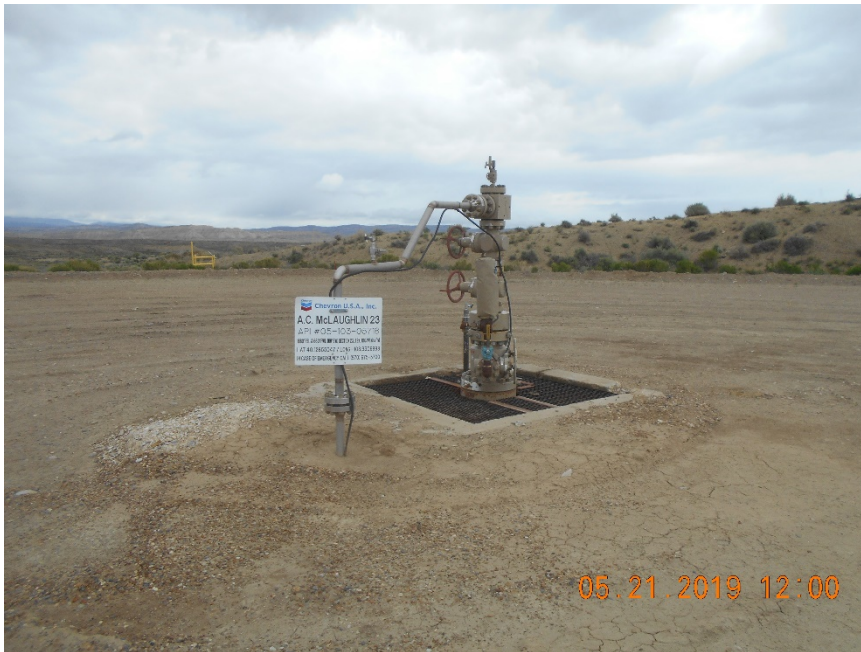
Injection wellhead
