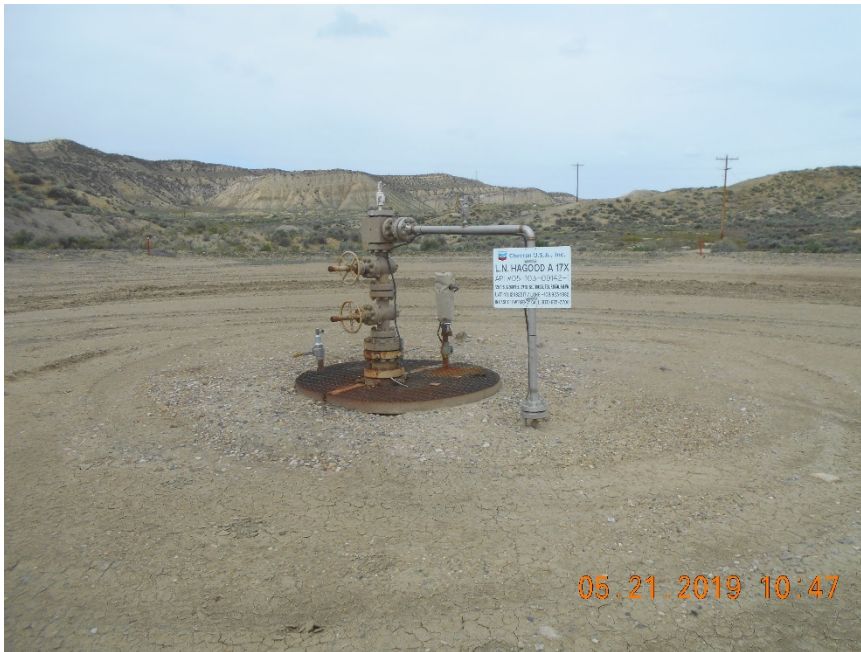
Injection wellhead
