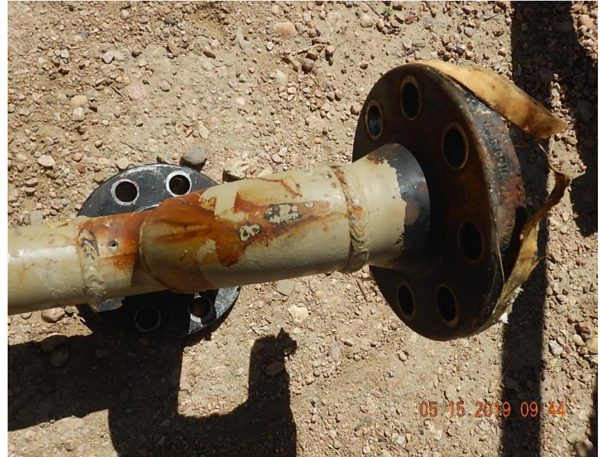
Process pipe assembly and corrosion pinhole.
