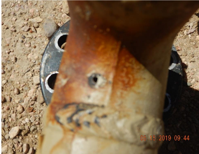
Corrosion pinhole resulting in release.
