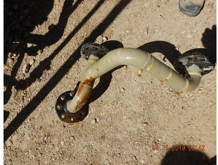
View of process pipe assembly/ equipment failure.
