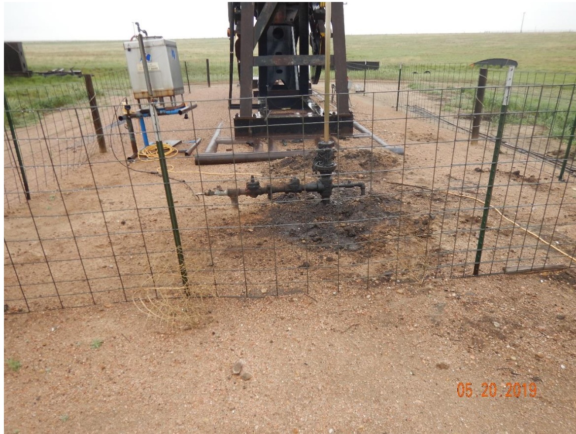
Photo 1: Photo taken from the well head, facing west. Photo shows stained soils have not been removed from the wellhead.
