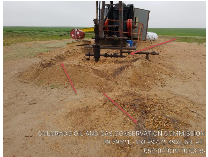
Pic 6 stained soil near wellhead
