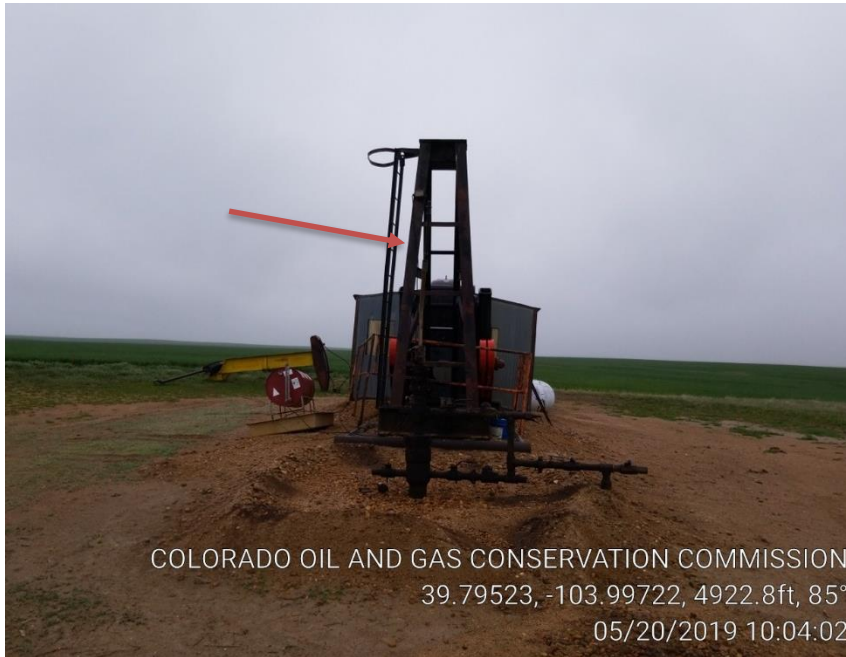
Pic 7 polish rod is bent, no horses head on pumping unit
