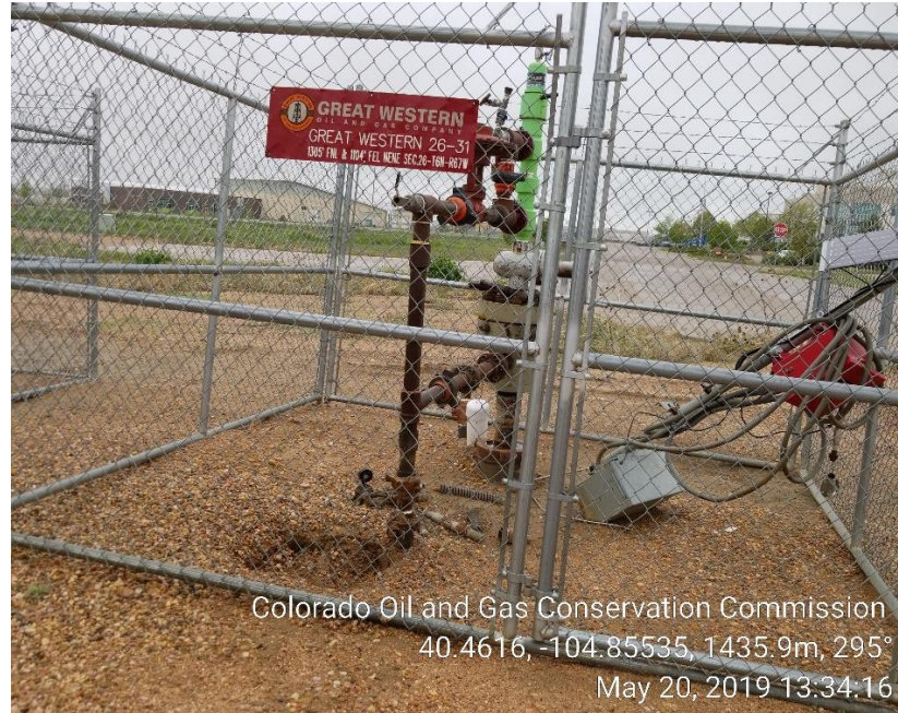
Photo 1: Wellhead; unused equipment, missing emergency contact #.
