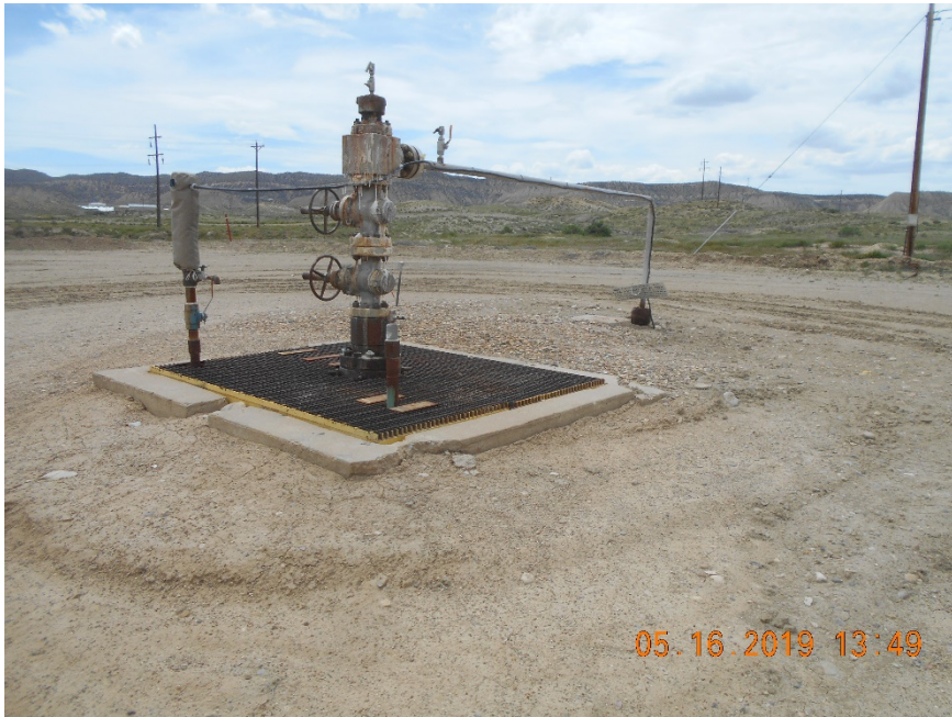
Injection wellhead
