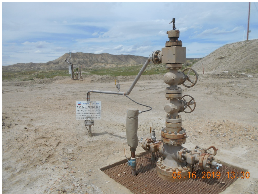
Injection wellhead
