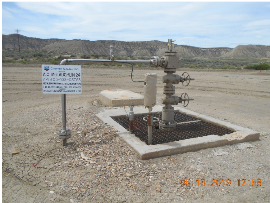
Injection wellhead
