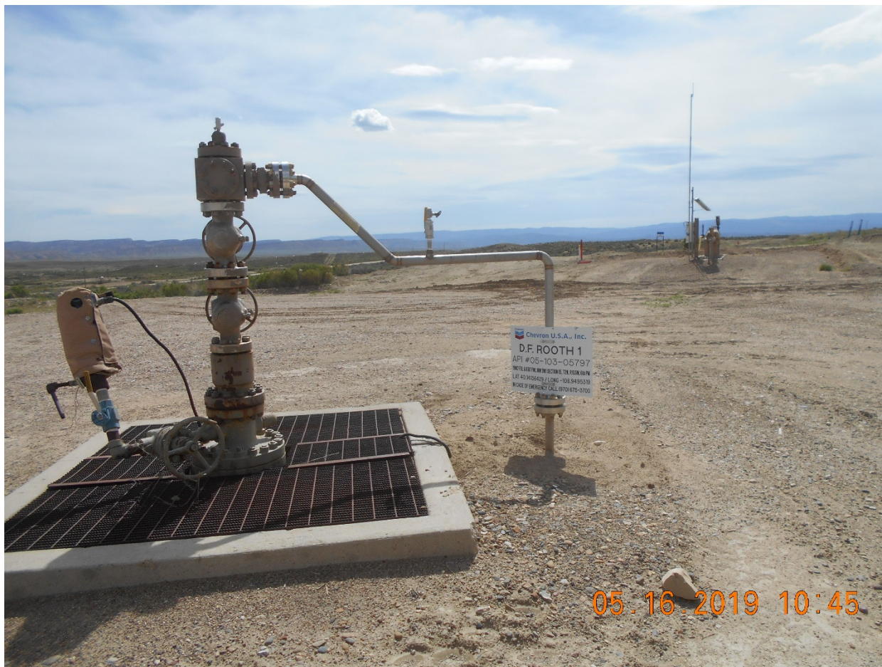
Injection wellhead with WAG skid in background
