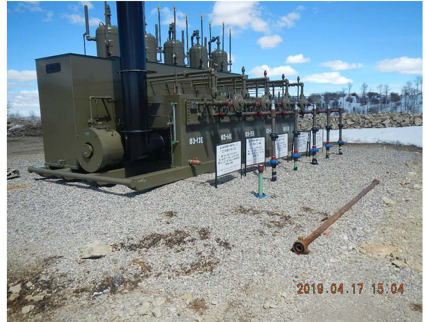
Oil stained soil, uncapped, unmarked riser.
