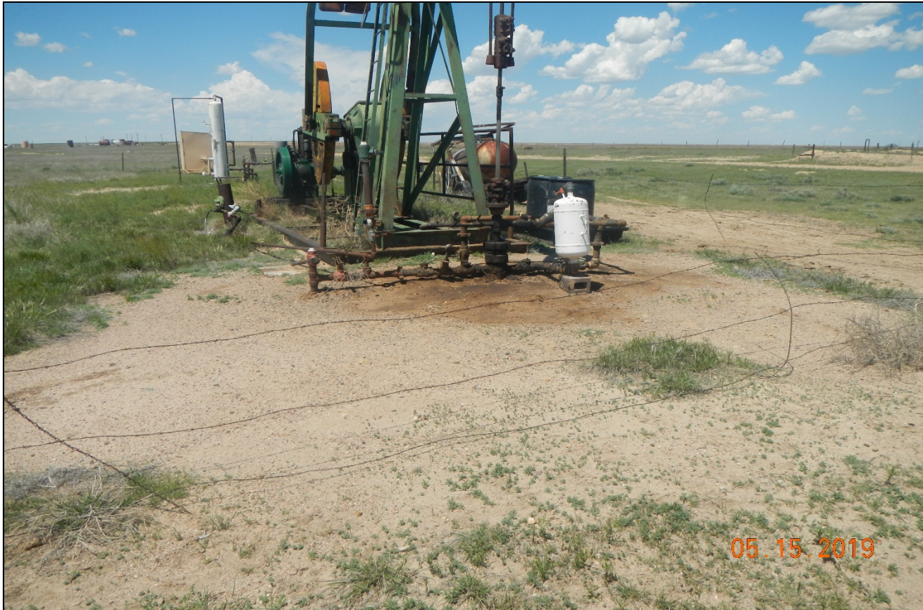
Photo 3. There is oil stain soil around the wellhead.
