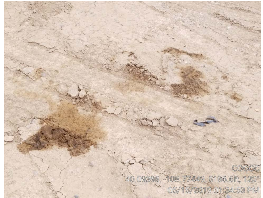
Photo 4. Oily waste at truck loading between tank battery and separator.
