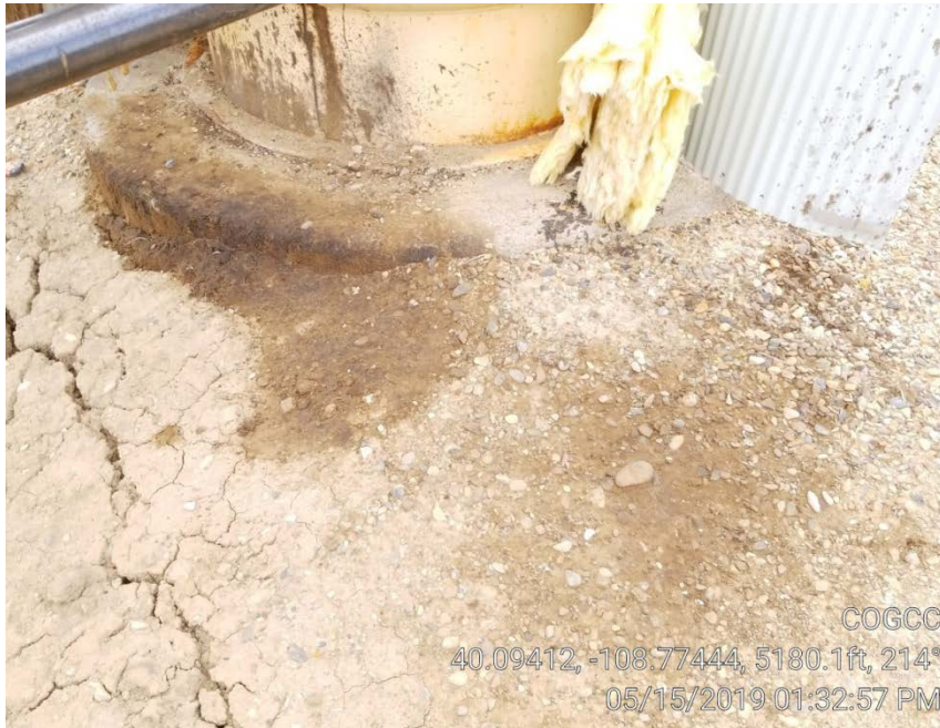
Photo 3. Oily waste next to vertical separator at tank battery.
