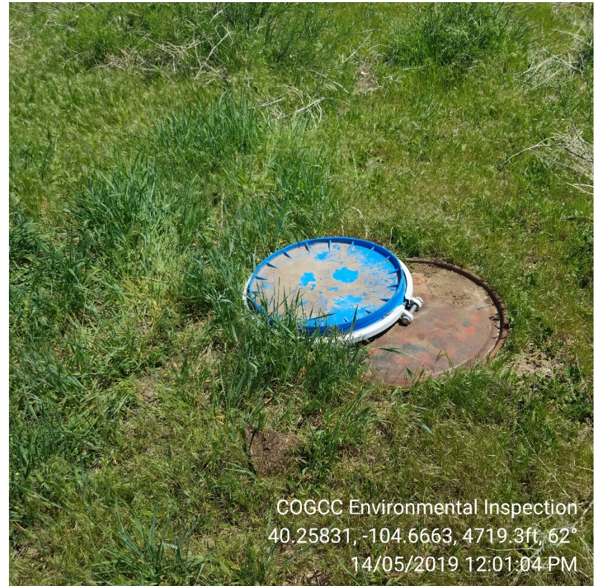
Photo 2 – Improperly abandoned soil boring (TH-04) remains unfilled and capped by scrap metal placed by COGCC on 4/24/2019.
