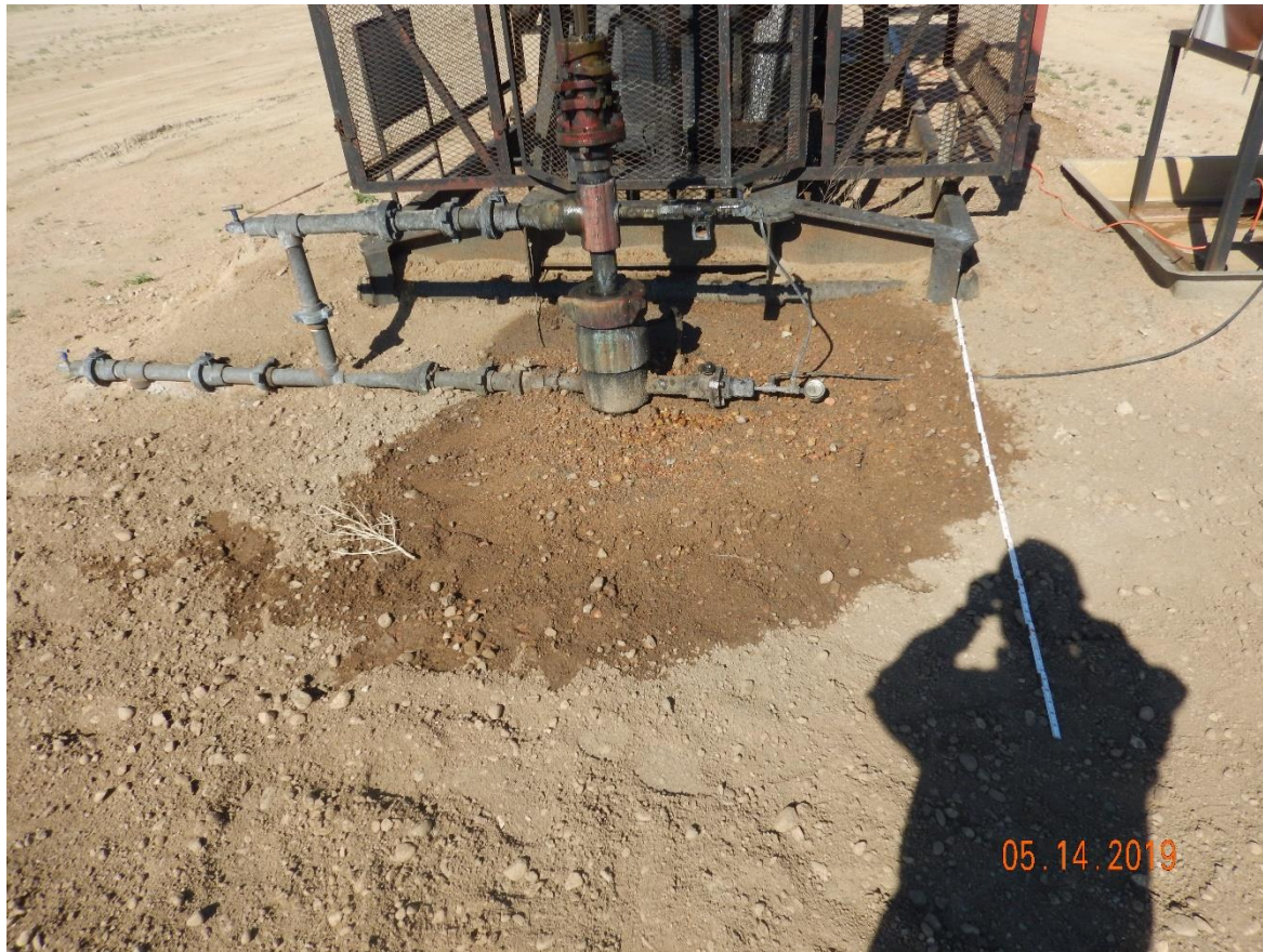
Photo 5: Continued from photo 3. Photo shows fluids observed discharging from the pump rod have re-contaminating approximately a 5 ft. x 6 ft. area at the well head. 6 foot measuring stick for reference.
