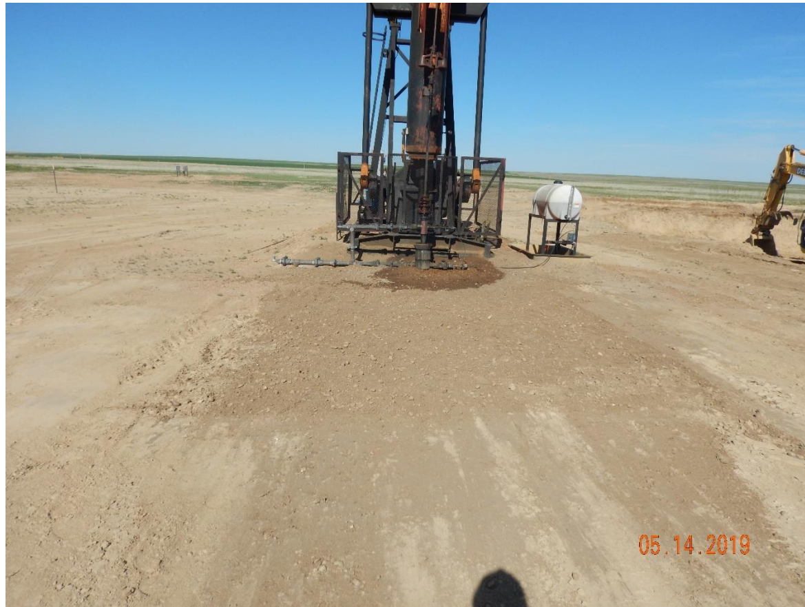
Photo 3: Photo taken from the well, facing west. Previous inspection documented a fluid spill at the wellhead. Operator was provided a 24 hour notices to control/contain fluid spill and clean up stained soils in accordance with 906.a. Photo shows stained soils appear to have been removed, however, Operator has failed to control/contain the fluid spill at the well head. Fluids were observed actively discharging from the pump rod contaminating approximately a 5 ft. x 6 ft. area at the well head.
