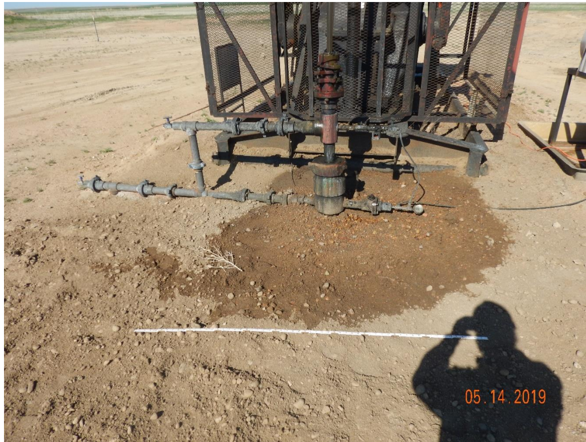
Photo 4: Continued from photo 3. Photo shows fluids observed discharging from the pump rod have re-contaminating approximately a 5 ft. x 6 ft. area at the well head. 6 foot measuring stick for reference.
