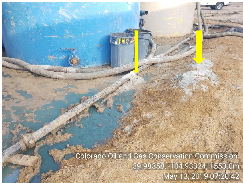
Photo 9 Spill release: unknown fluid in drill out tank containment. Frac sand in and on berm. Inadequate containment.
