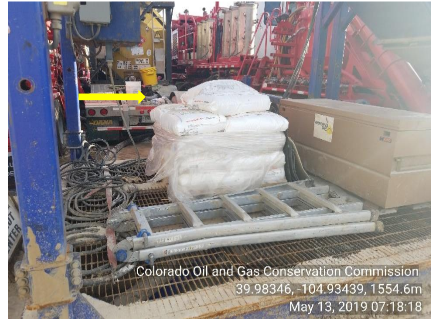
Photo 6 Improper chemical storage: Chemical's not covered.
