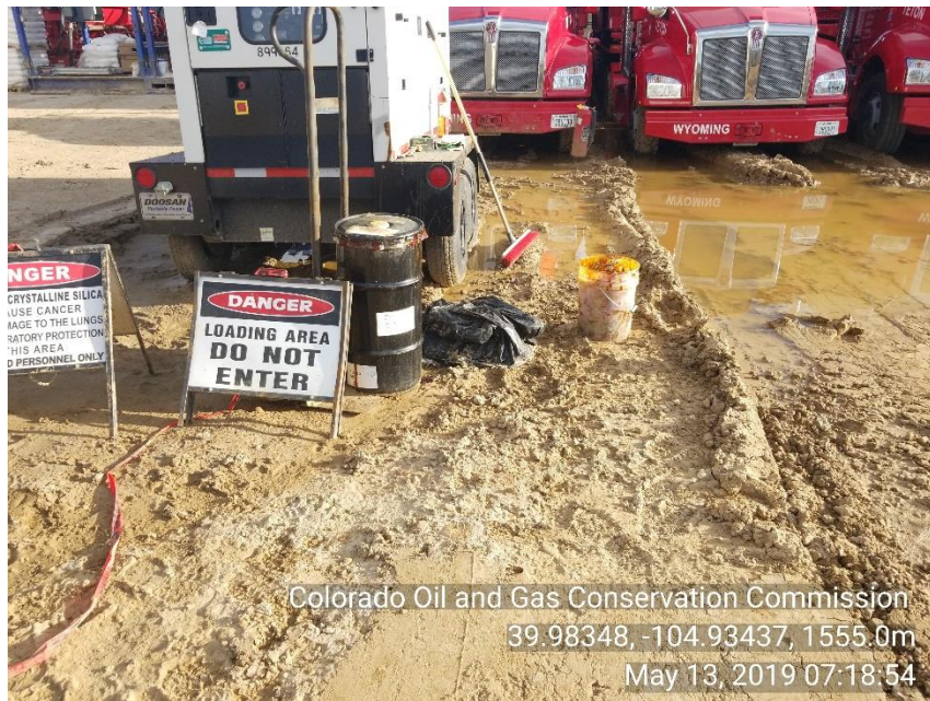
Photo 7 Improper storage of grease. No secondary containment.
