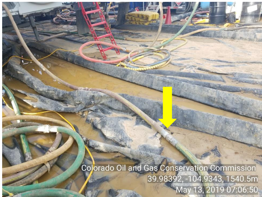
Photo 3 Chemical hose cam lock not properly taped or double lock cam lock
