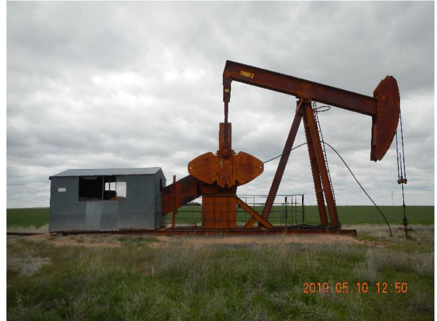
Photo 2: Pump jack and prime mover shed.
