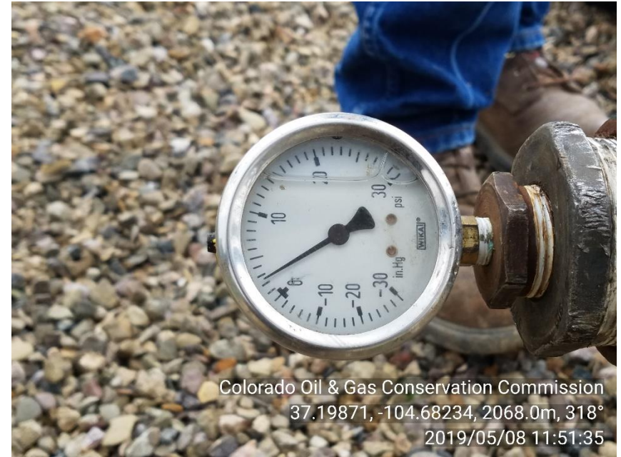
PHOTO 4: CASING PSI AT 3.5 PSI AND HELD THROUGHOUT THE TEST
