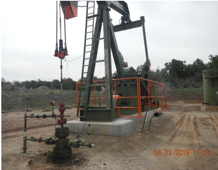
IGE #140 pump jack with stained soil around wellhead.
