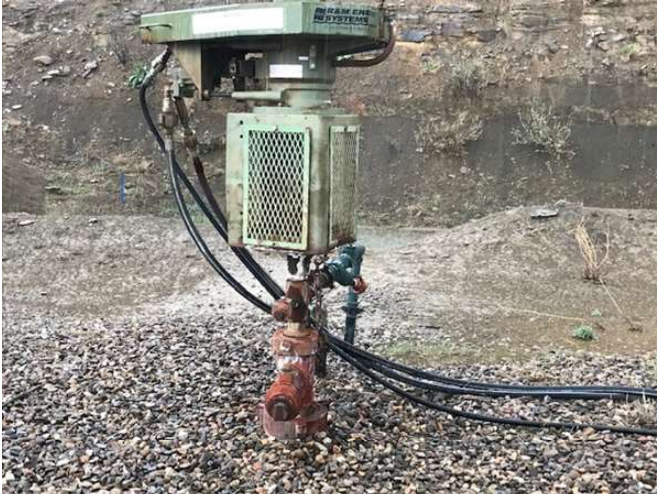
PHOTO 1: THE IMPACTED SOIL AROUND THE WELL HEAD WAS CLEANED UP AND REMOVED FROM THE LOCATION. ALL VALVES AND FITTINGS WERE SECURELY FASTENED ON 04/12/19 TO STOP THE LEAKING PACKINGS.
