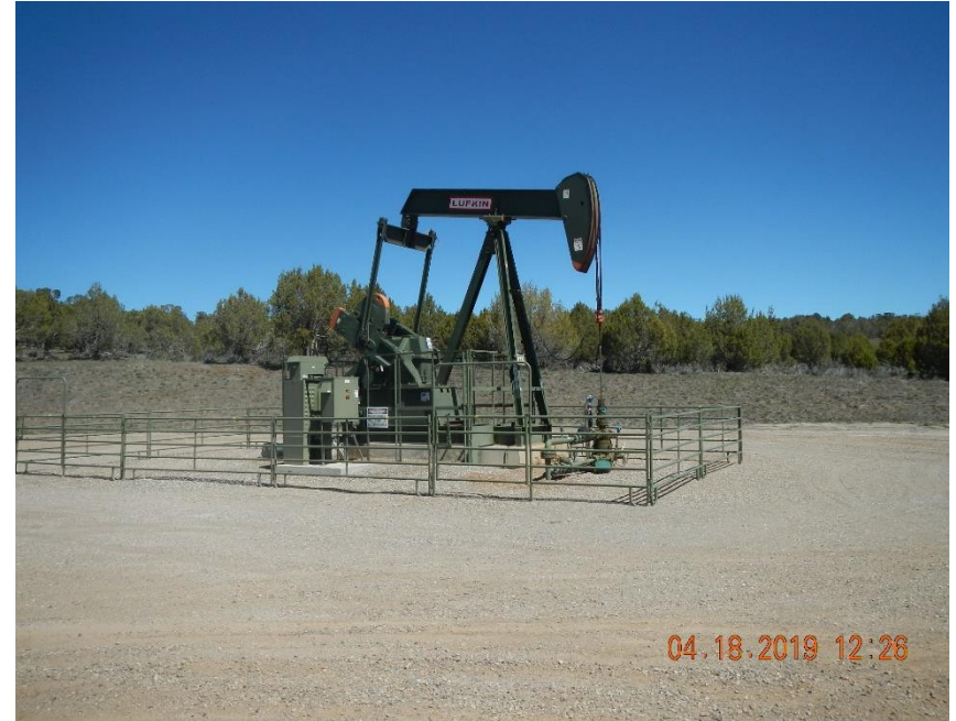
McCaw 34-15 #4 wellhead and pump jack with electric motor.
