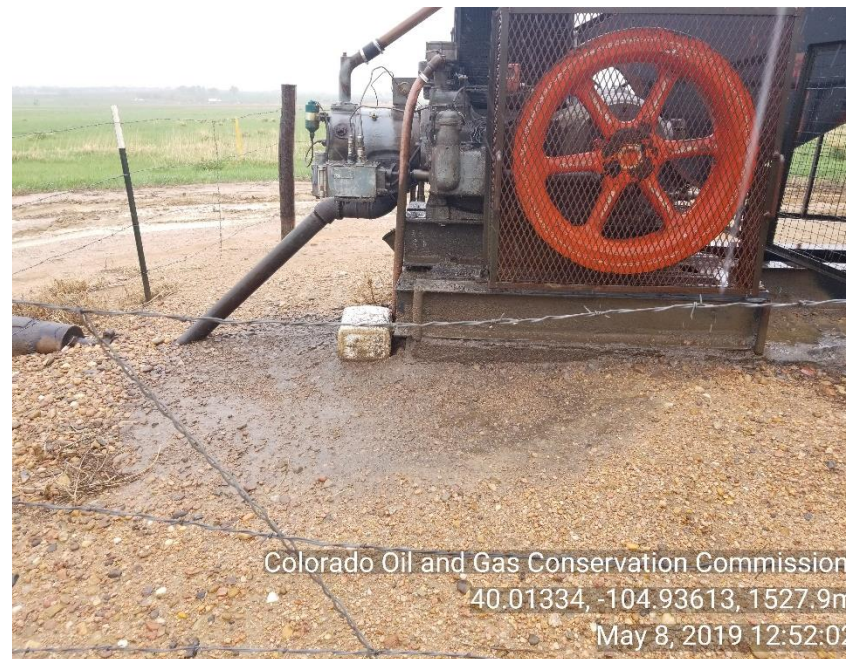
Photo 2 Stained soil around PU motor
