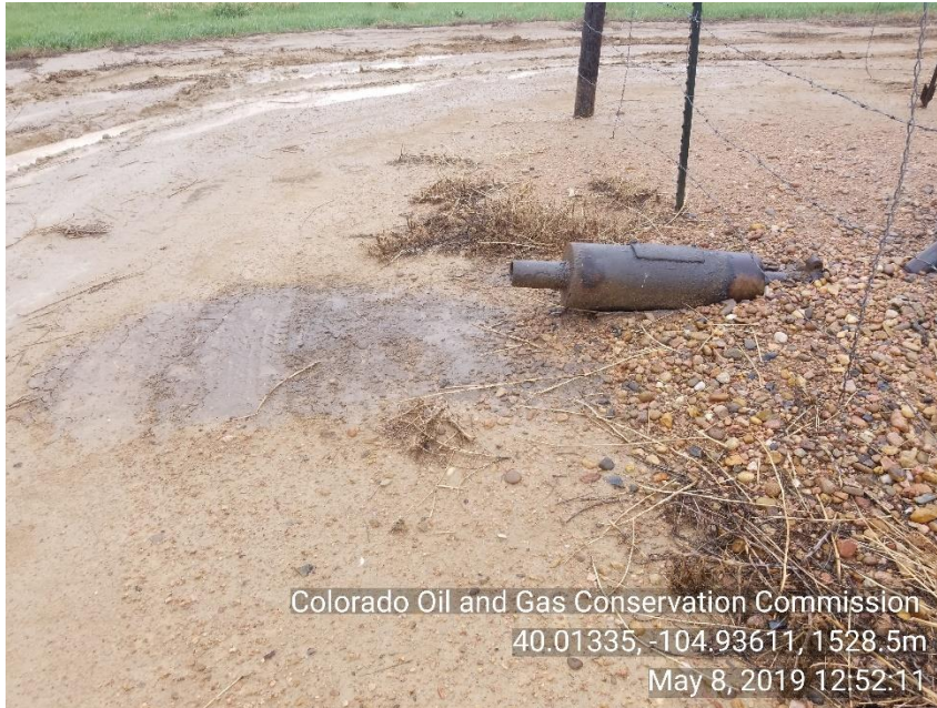
Photo 3 Stained soil around exhaust pipe for PU motor
