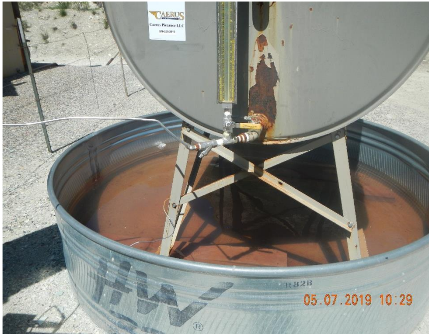
Photo 3 Secondary containment is full of fluid.
