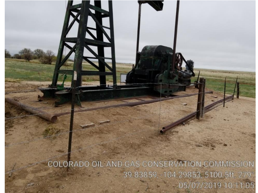
Pic 4 unused tubing and rods, stained soil.
