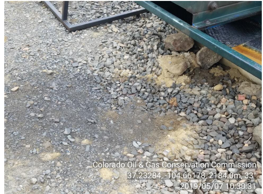
PHOTO 8: IMPACTED SOIL ON WEST SIDE OF ENGINE SKID. Securely fasten all valves, pipes, and fittings to ensure good mechanical condition, inspect at regular intervals and maintain in good mechanical condition per Rule 605.d. Non E&P Waste not properly stored, handled, transported, treated, or disposed per Rule 907A. CA DATE 6/7/19
