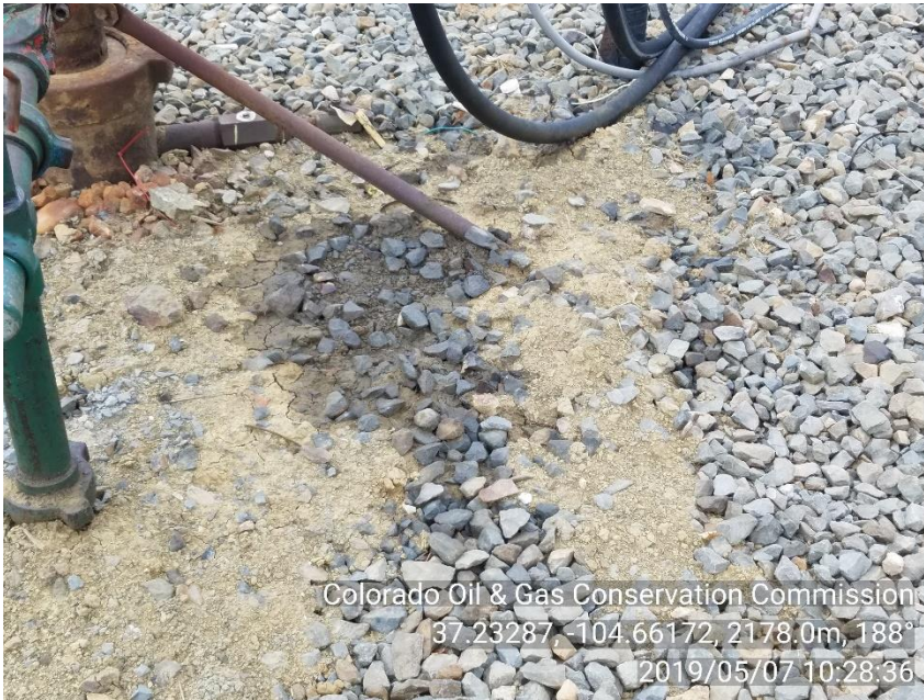
PHOTO 7: IMPACTED SOIL NEXT TO WELLHEAD BENEATH DRIVEHEAD MOTOR. Securely fasten all valves, pipes, and fittings to ensure good mechanical condition, inspect at regular intervals and maintain in good mechanical condition per Rule 605.d. Non E&P Waste not properly stored, handled, transported, treated, or disposed per Rule 907A. CA DATE 6/7/19
