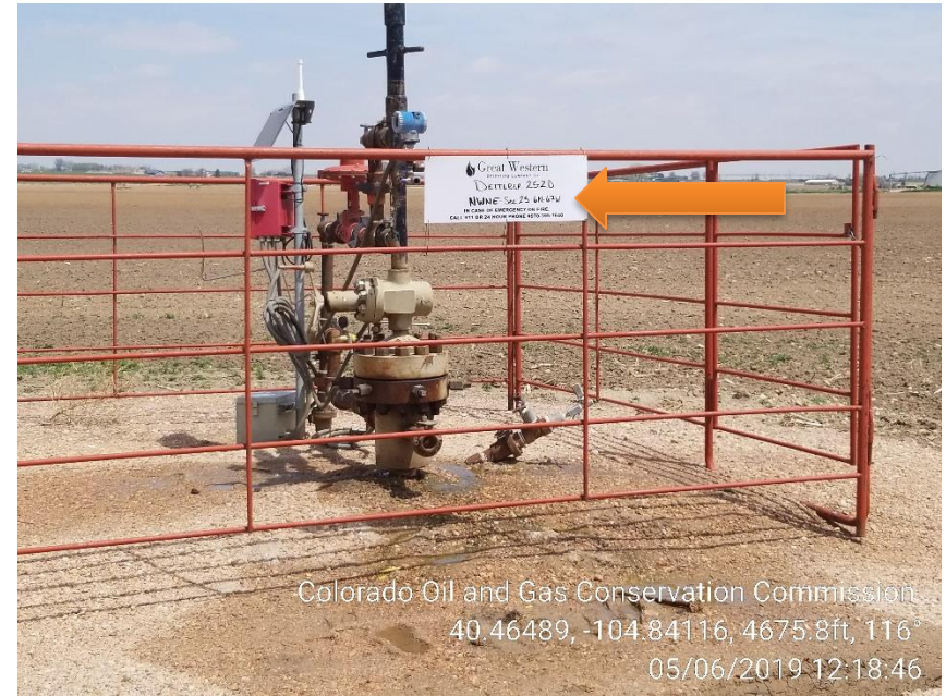
Photo 4 – Wellhead Signage is incorrect.
