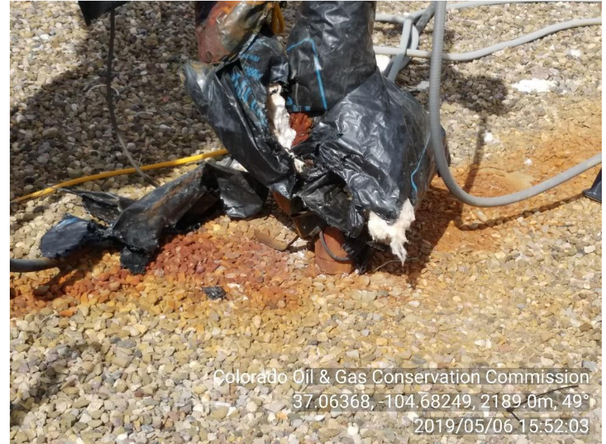
PHOTO 4: IMPACTED SOIL NEAR WELLHEAD NO LEAK OBSERVED AT TIME OF INSPECTION Comply with Rule 603.f .
