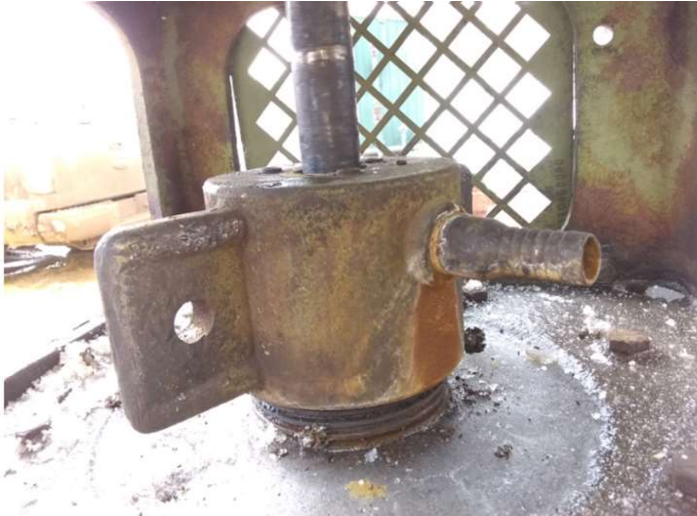
PHOTO 1: REPLACED THE PACKING TO ELIMINATE THE WATER LEAK. PACKINGS WERE SECURELY FASTENED.
