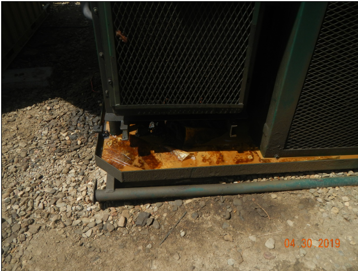
Photo 5. There is oily waste in the engine skid.
