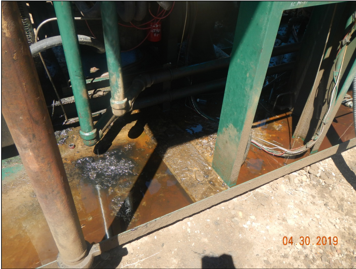
Photo 3. There is oily waste at the engine skid.
