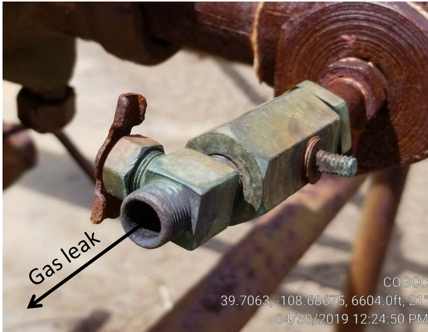
Photo 2. Gas leak at well head.
