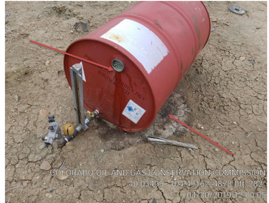
Pic 2 chemical barrel appears to be leaking. No containment.
