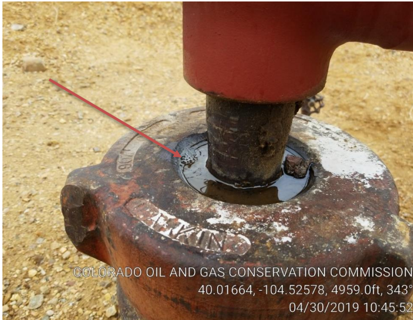
Pic 3 possible leak.
