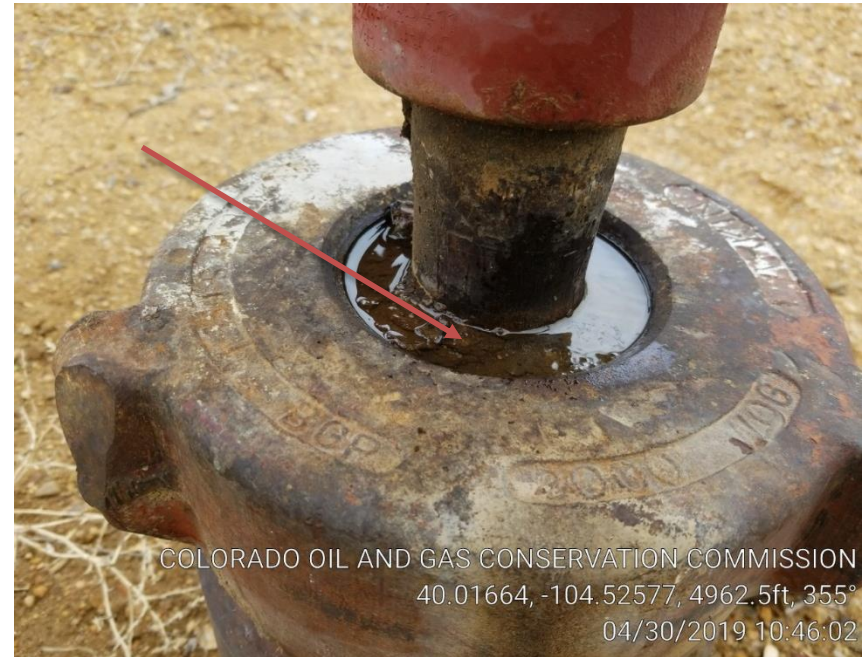
Pic 4 possible leak.
