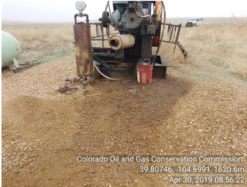
Photo 7 Stained soil around PU motor. Trash: 5 gallon bucket.
