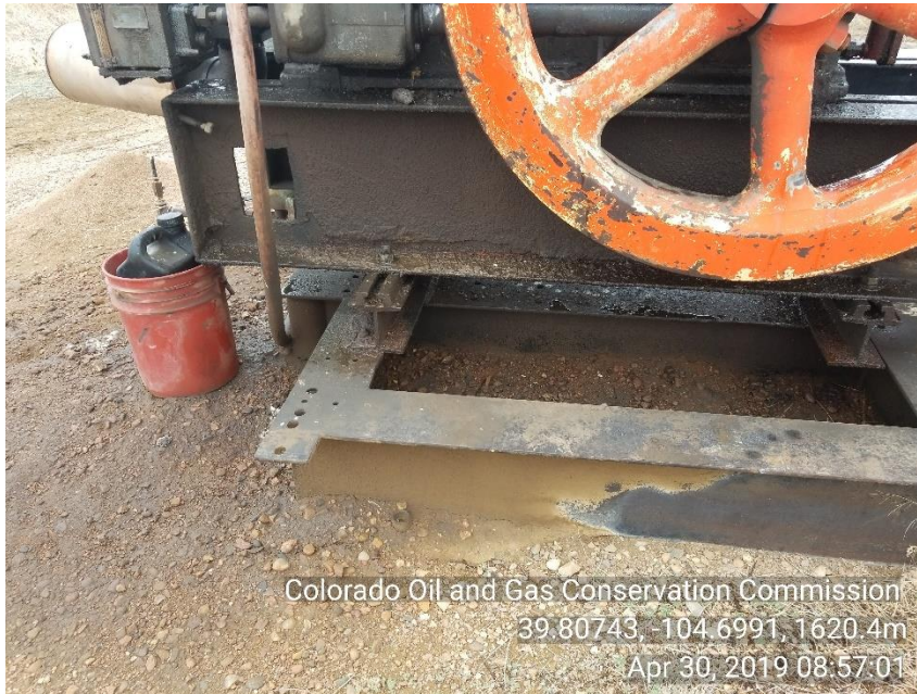
Photo 9 Stained soil around PU motor. Trash: 5 gallon bucket.
