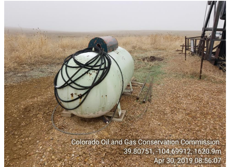
Photo 6 Unused equipment: propane tank and sucker rods.
