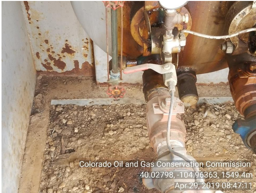
Photo 3 Mechanical issue: inside separator house appears piping to separator is leaking.
