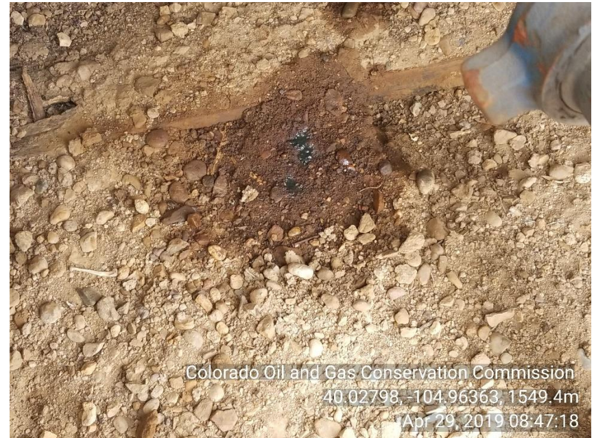
Photo 4 stained soil under what appears to be leaking piping to separator.
