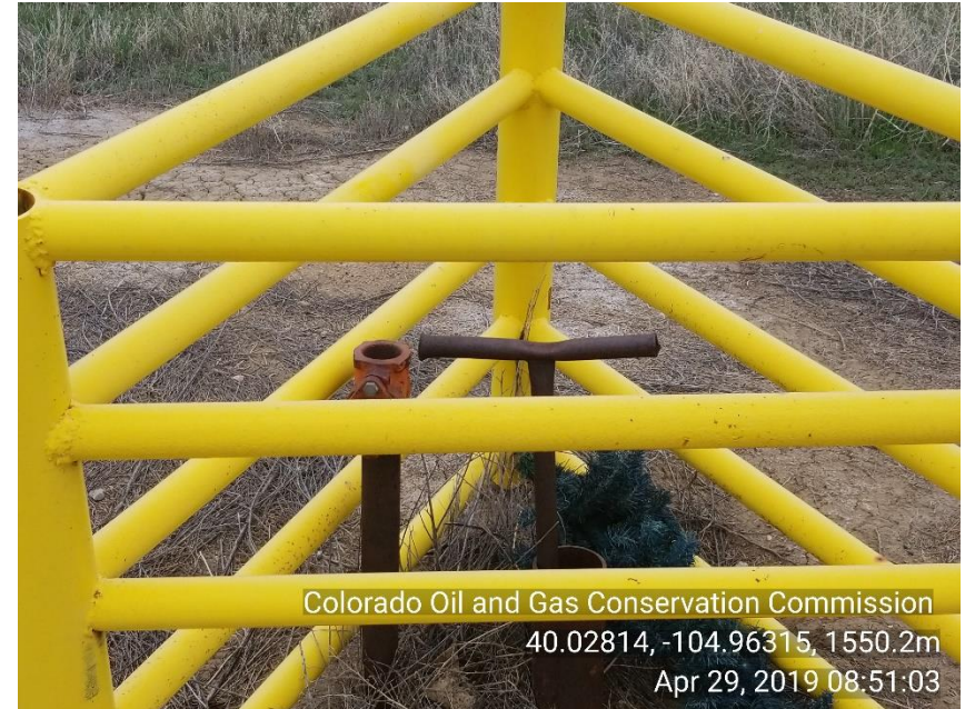
Photo 6 Unused, unmarked not LOTO or bull plugged riser.
