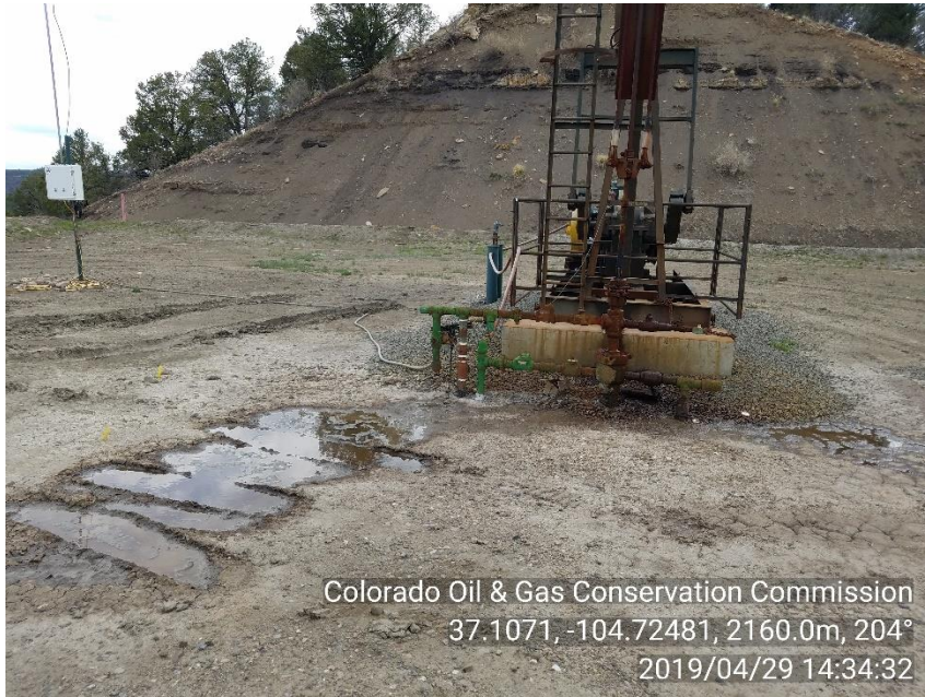
PHOTO 3: ROD PACKING IS LEAKING PRODUCED WATER
