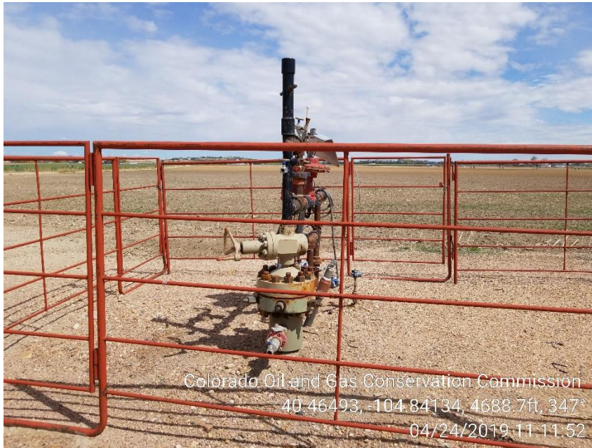
Photo 3 – Well Detterer FD 25-6D, API 123-35571, missing wellhead signage.
