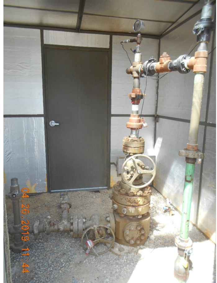
Injection wellhead
