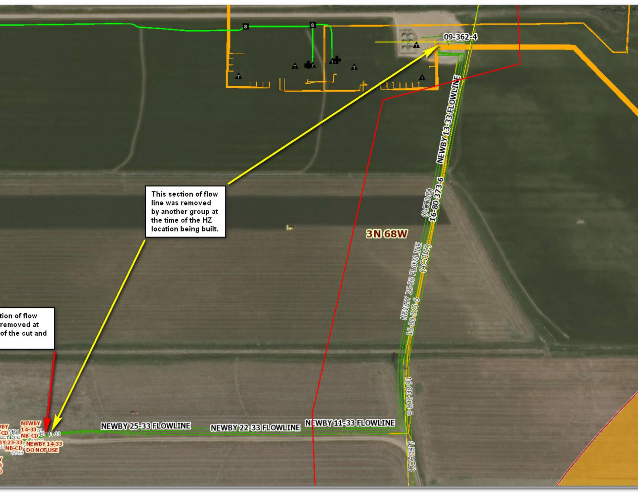
This section of flow line was removed by another group at the time of the HZ location being built.
